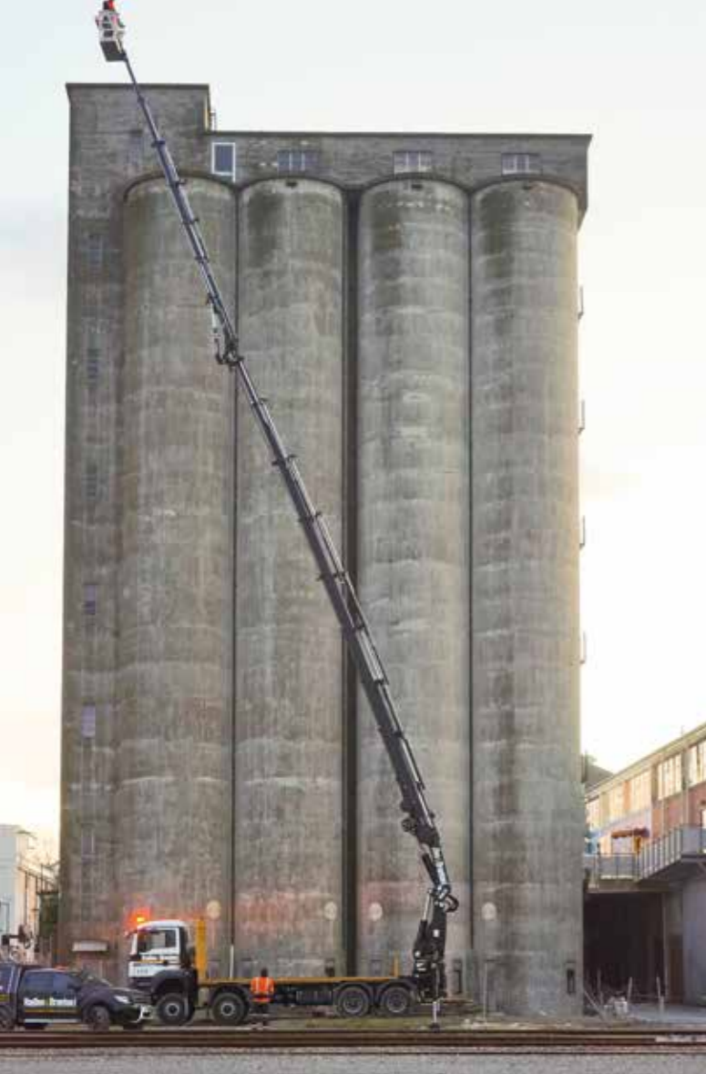
The spectacular reach of the HIAB XS544 E-8 crane fitted to the company's MAN 8x8 is clearly demonstrated in these pictures. On major projects the MAN supplies drilling pipe to the rigs, but it has a myriad of other uses. All-wheel-drive offers real benefits offroad
