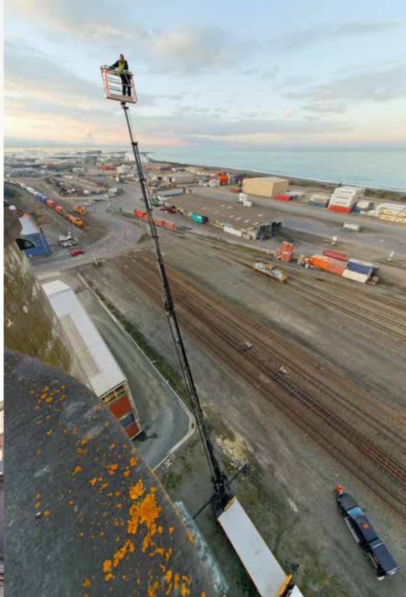
The spectacular reach of the HIAB XS544 E-8 crane fitted to the company's MAN 8x8 is clearly demonstrated in these pictures. On major projects the MAN supplies drilling pipe to the rigs, but it has a myriad of other uses. All-wheel-drive offers real benefits offroad
